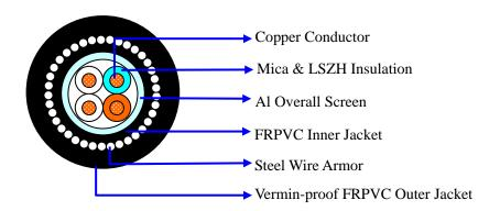
**Conductor:** Plain Annealed Solid Copper to IEC 228 Class 1
